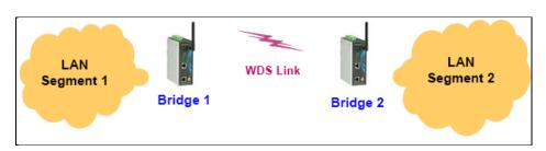
It is a good idea to plan your wireless network by drawing a diagram so that you know how each AWK-3131A is connected to other peer APs or wireless bridges by WDS, and how bridges are connected to other peer bridges by WDS. See the following figure for an example of a network-planning diagram.
