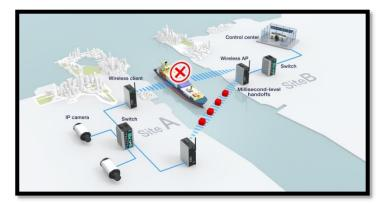
2. **Frequency-Interference Failover:** This concept is similar to the previous model. If the communication frequency experiences interference and data can no longer be transmitted over the Active frequency, it will resume the connection via another Backup frequency.
