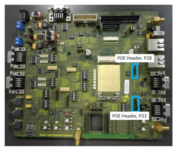
The development board provides two PoE module connectors, P28 and P33, to plug a Digi PoE module (DG-ACC-POE). The PoE module is an optional accessory item that can be plugged on the development board through the two connectors.
