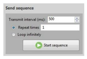
Click Start sequence. XCTU sends all frames in the Send frames list. Sent and received frames appear in the Frame logs area.
