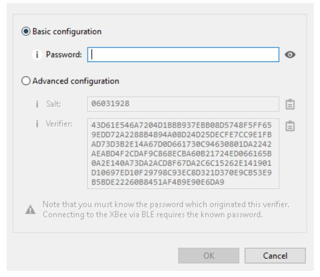
When you enter the password or the salt/verifier combination, click **OK** to save the settings to the module.
