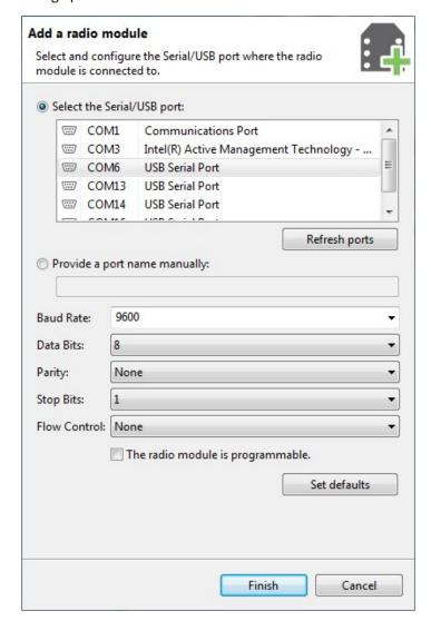
2. Select the serial port where the radio module is connected (or enter its name manually) and configure the serial settings of the port.
