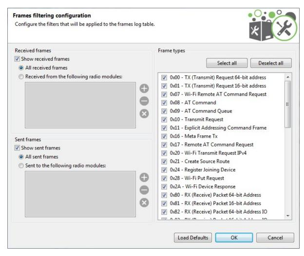
4. Configure the filtering options for one or more of the following: received frames, sent frames, and frame types.
