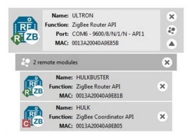
**Note** XBee Wi-Fi modules do not support the remote radio modules discovery feature. Instead, they can look for access points.
