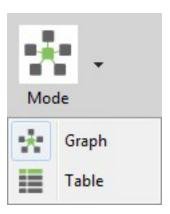
In Table view, network radio modules are displayed as rows in a table. ZigBee devices display end devices as children of their coordinators or routers. Other protocols display all nodes at the same level.
