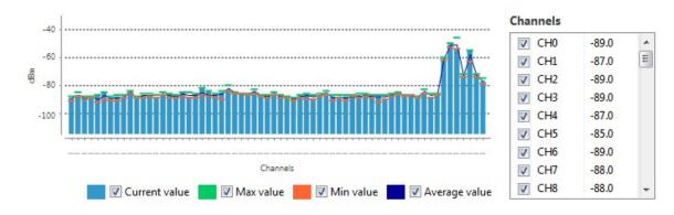
5. Use chart filters to hide or display channels, the best and worst noise level values and the average noise level line. You can also display channel values and samples read. For details, see Spectrum analyzer tool.
