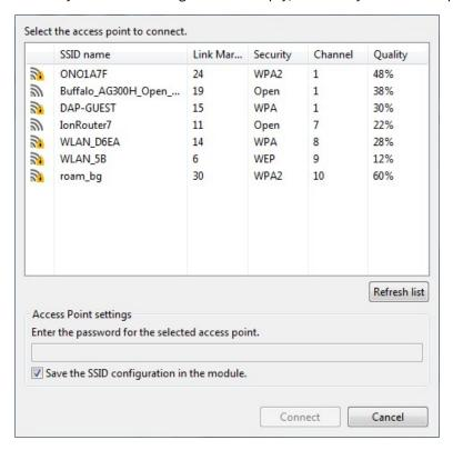
The dialog displays all the nearby access points as well as their security protocols and signal quality. Select the Access Point you want the Wi-Fi module to connect to and, if necessary, configure the password of the Access Point. The Access Point settings also have a check box that allows you to permanently save the SSID configuration in the Wi-Fi module. If you uncheck this option, the next time you reset the module the SSID configuration is cleared.
