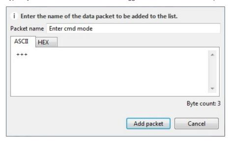
4. Click **Add packet**. The data packet appears in the list of packets. Repeat the operation to add additional packets to the list.
