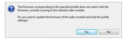
If the firmware of the configuration profile is not compatible with the radio module, click Yes to open the profile in the Profile editor tool.
