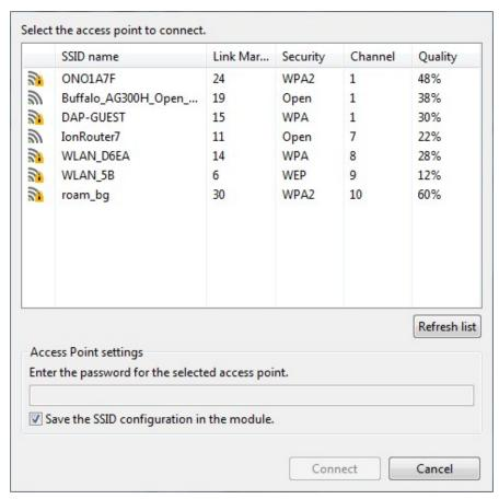
4. Select the SSID you want the Wi-Fi module to connect to. For S6 Wi-Fi modules, the table displays the following fields:
