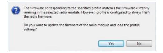
■ If the firmware of the profile you are loading and the firmware running in the radio module match or the profile is configured to don't flash the radio firmware, XCTU applies the settings saved in the profile to the radio module.
