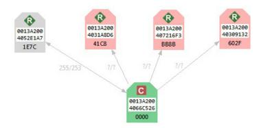
Red radio modules represent devices that were in the network at any time in the past but are unreachable now. When a radio module leaves the network, some devices may still contain information about it. When a new discovery is performed, the module appears to be there but does not answer or is unreachable when XCTU tries to verify the connection.
