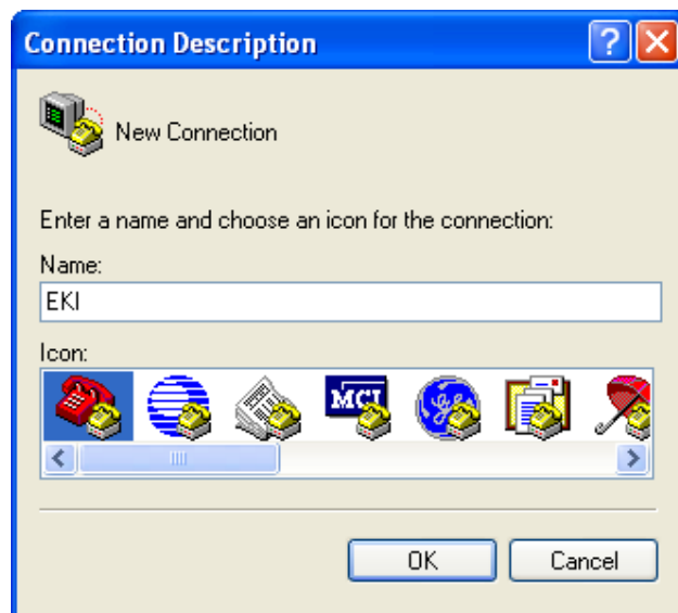
Figure 7.1 Creating a Telnet Connection
