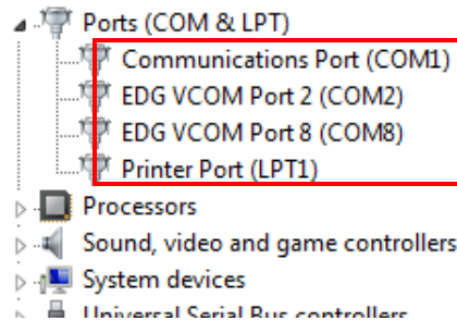
Figure 5.10 System Port VCOM Mapping Configuration
