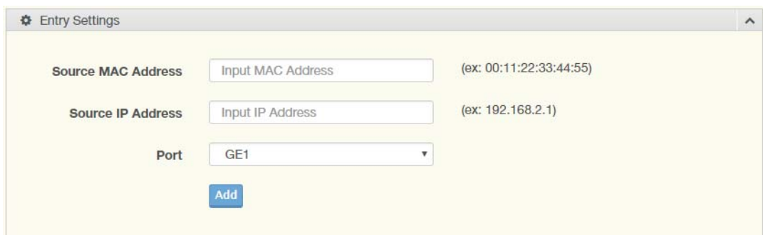
Figure 4.81 Security > IP Source Guard > Entry Settings
