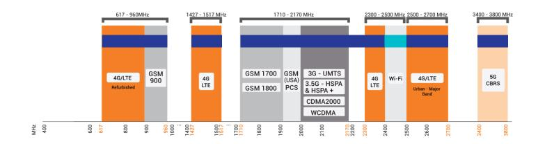
Indicates the 5G/LTE bands on which OMNI-85 works
