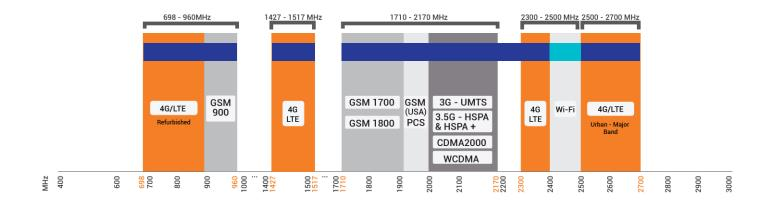
Indicates the LTE bands on which OMNI-121 works
