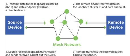
The configuration steps for sending data to the loopback cluster ID depend on what mode the device is in. For details on setting the mode, see AP (API Enable). The following sections list the steps based on the device's mode.
