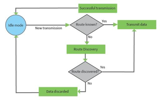
When DigiMesh data is transmitted from one node to another, the destination node transmits a network-level acknowledgment back across the established route to the source node. This acknowledgment packet indicates to the source node that the destination node received the data packet. If the source node does not receive a network acknowledgment, it retransmits the data.
