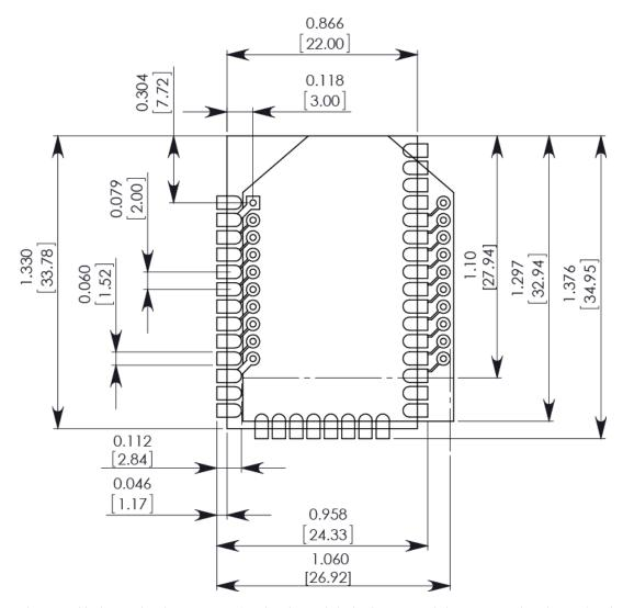
The round holes in the diagram are for the through-hole design, and the semi-oval pads are for the surface-mount design. Pin 1 of the through-hole design lines up with pad 1 of the surface-mount design, but the pins are actually offset by one pad (see Pin mapping). By using diagonal traces to connect the appropriate pins, the layout works for both modules.
