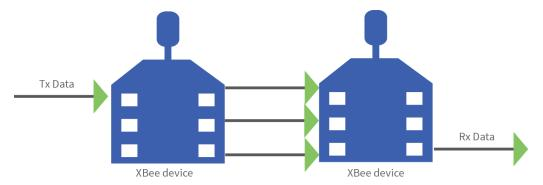
The transmit frame can include up to 255 bytes of data broken up into multiple transmissions and reassembled on the receiving side. If one or more of the fragmented messages are not received by the receiving device, it drops the entire message, and the sender indicates a transmission failure in Transmit Status frame - 0x8B.
