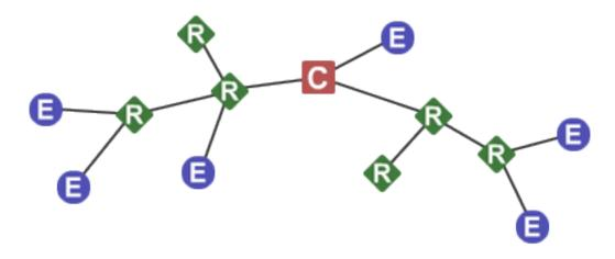
**Note** Each Zigbee network must be formed by one, and only one, coordinator and at least one other device (router or end device).
