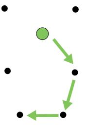
A remote device sends an RF data packet to the data collector. This is prefaced by a route record transmission to the data collector.
