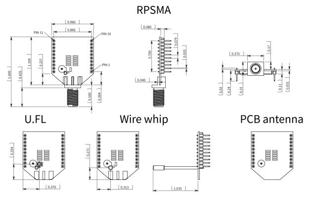
The drawings below show the XBee-PRO through-hole model.
