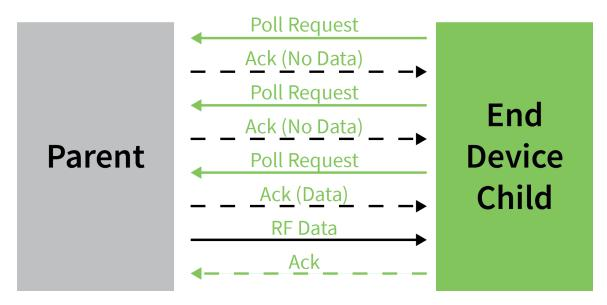
If the end device receives the acknowledgment and finds that the parent has no data for it, the end device can return to idle mode or sleep. Otherwise, it remains awake to receive the data. This polling mechanism allows the end device to enter idle mode and turn its receiver off when RF data is not expected in order to reduce current consumption and conserve battery life.
