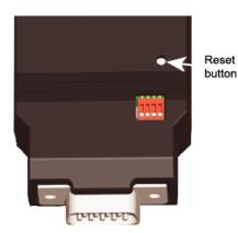
For Digi Connect EM or Digi Connect Wi-EM, the Reset button is located between P3 and CR1, as shown:
