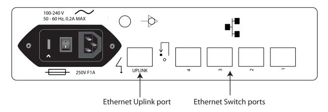
Because the LANs attached to each Digi Connect ES 4/8 SB with Switch are typically not connected to each other, equipment can have static network addresses and be moved from one location to another without needing to be reconfigured. The central data management system can easily communicate with the equipment by addressing the appropriate Digi Connect ES 4/8 SB with Switch device. The Digi Connect ES 4/8 SB with Switch uses NAT and port forwarding to make the connection.
