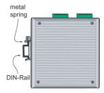
To remove the EDS-510A from the DIN-Rail, simply reverse Steps 1 and 2 above.
