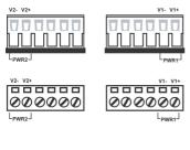
**STEP 1**: Insert the negative/positive DC wires into the V-/V+ terminals, respectively.
