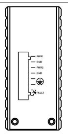
Field Wiring Terminal: Use Copper Conductors Only,  $60/75^\circ\!\!\mathbb{C}\,,~12\text{-}24$  AWG torque value 7 lb-in.
