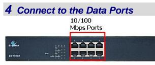
The switch is equipped with eight 10/100 Mbps RJ-45 port that provide IEEE802.3at Power over Ethernet (PoE), with up to 30 Watts per port (50 - 57VDC, 600mA Max.) These ports can be connected to PoE devices such as IP surveillance cameras or Voice Over Internet Protocol (VoIP) phones.
