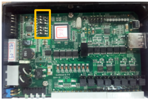
*Default setting (high/low resistors to 150 KΩ)
