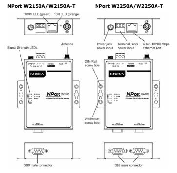
**Reset Button**: The reset button is used to load the factory default settings. Use a pointed object to hold the reset button down for five seconds to load the factory defaults.
